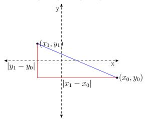
The line segment that determines the distance between the points is the hypotenuse of a right triangle with legs of length  $|x_1 - x_0|$  and  $|y_1 - y_0|$ . If D denotes the distance between  $P_0$  and  $P_1$ ,
