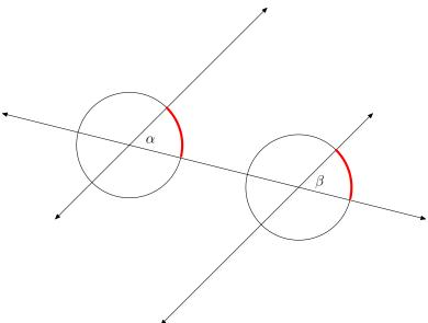
Each angle cuts off an arc. It is visually obvious that the lengths of these arcs are equal. As a consequence, these angles are congruent:  $\alpha = \beta$ . The general principle: alternating angles are congruent.
